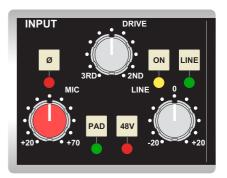
Both of these preamps use the same gain control providing +20dB to +70dB gain and share a passive front end with a switchable 22dB Input Pad and +48V phantom powering.
